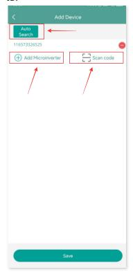
4. The search result of microinverters and microinverters added will be displayed in the list. Tap the button on the right if you want to delete it.
