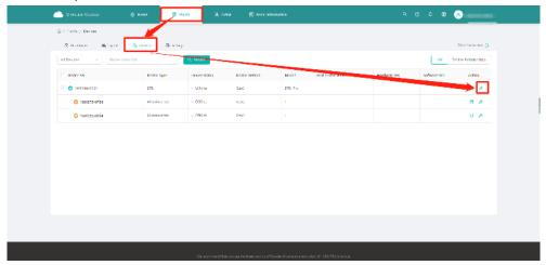
3. Click "Replace Device", enter the current device SN and click "OK" to complete DTU replacement.
