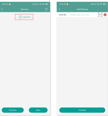
6. Scan or input the microinverter ID. Press "Finish" when all microinverter IDs have been input.
