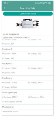
Note: If the microinverter signal is so weak that the real-time data are not updated, move the DTU closer to the microinverter.
