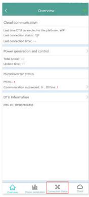
2. On this page, you can check the signal strength between the DTU and each microinverter. Tap the signal icon to enter the respective microinverter page (signal quality is constantly refreshed).
