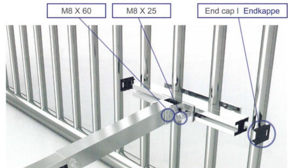
4.15 L foot installation and connection: The L foot is locked on the other side of the panel frame with bolts, and then connected with the telescopic rod with bolts;
