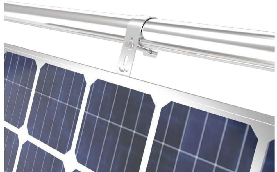
4.13 Rail installation: The bolt head snaps into the groove of the rail, the aluminum plate is on the other side of the railing, and the bolt is locked as shown in the picture;
